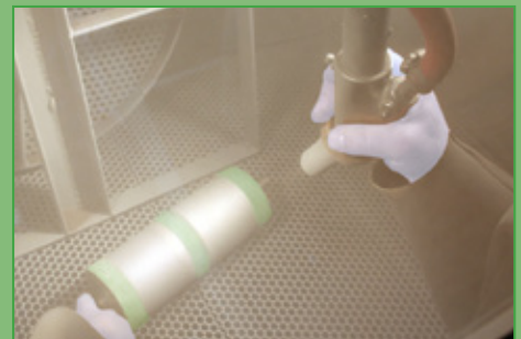
Grit blasting prepares the surface to receive the HVOF spray coating. Masking also protects the part from the grit blast particles.
