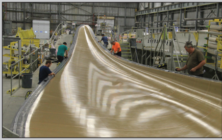
Application of PTFE mould release can be consistent from root to tip..
