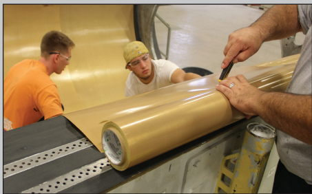
GR6 Mould Release is a premium reinforced PTFE product developed for the wind blade market.
