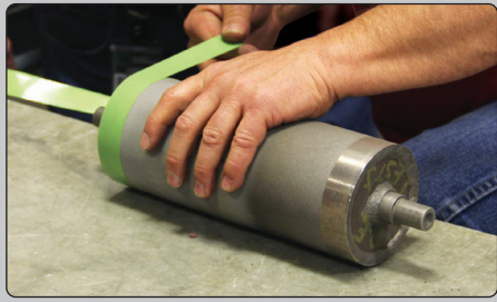
170-10S Green applied to cylinder prior to grit blast and thermal spray coating.
