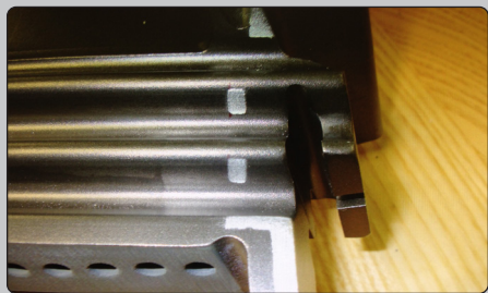
The same part is shown above, after receiving the spray coating.
