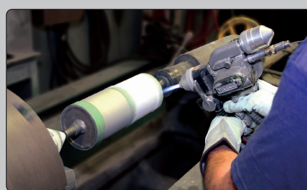
Flame spray coating applied to a component masked with 170-10S Green.
