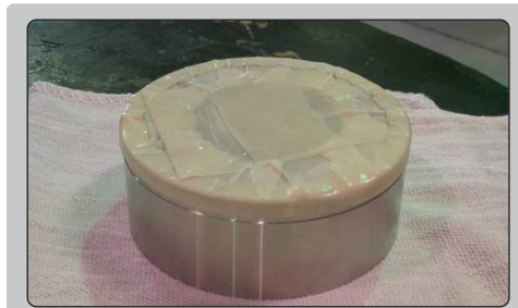
A part masked with multiple layers of tape.
