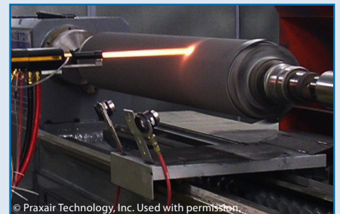
LF-HVOF spray coating being applied to a rotating cylindrical part.
