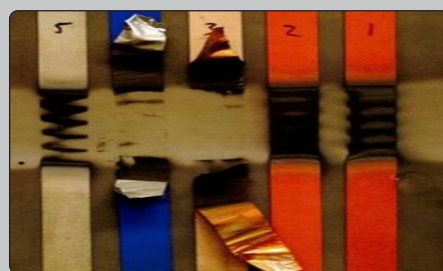
Ineffective masking tape can fail under the heat and abrasion of thermal spray coating processes.
