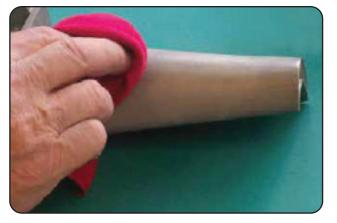
Before applying tape, remove dust, grease and dirt with a cloth and alcohol, or tack cloth.
