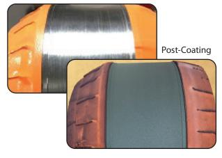
Properly applied, HVMT Orange tape will protect non-target surfaces from the extreme heat of the coating process.
