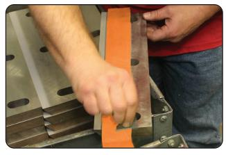
Apply tape and remove ripples, air pockets and bubbles with a smoothing tool.
