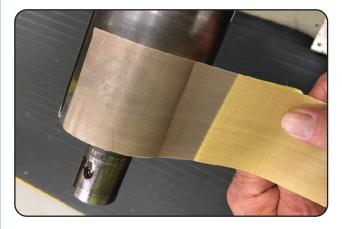
Carefully remove liner while smooth across surface, avoiding wrinkles and removing any bubbles.
