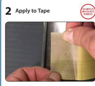
Remove approximately 2 inches of liner and apply to surface.
