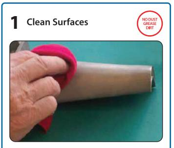
Before applying tape, remove dust, grease and dirt with a cloth and alcohol, or tack cloth.
