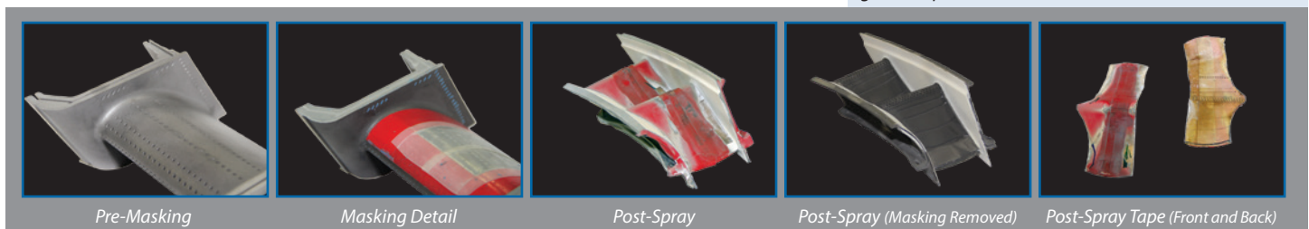
Grit blasting prepares the surface to receive the HVOF spray coating. Masking also protects the part from the grit blast particles.
