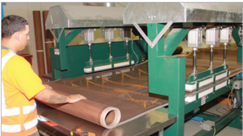
PTFE / Glass fabric edges are heat-sealed on a mesh dryer belt.
