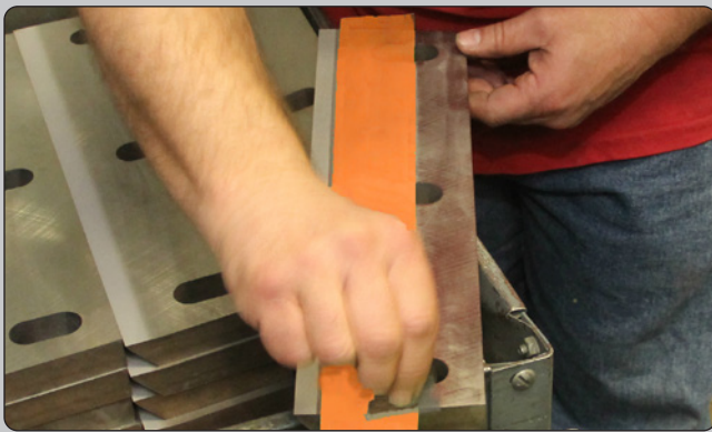
Applying HVMT Orange Masking Tape to a plate prior to receiving GF-HVOF Coating.
