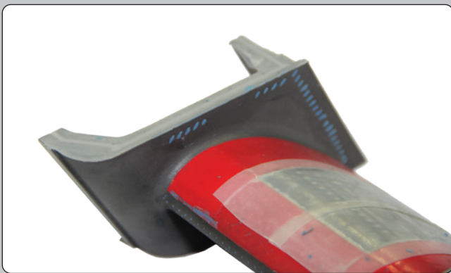
170-10S (Red) and High Velocity Masking Compound (Blue) provides primary masking and 160-5S (White) Masking Tapes is used for secondary masking on this turbine blade.
