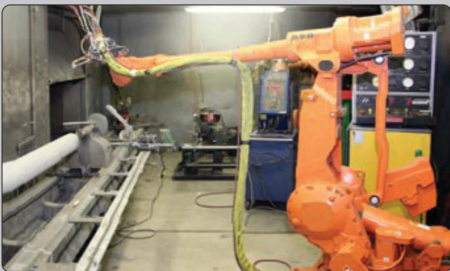
Robots are often used to apply thermal spray coatings.
