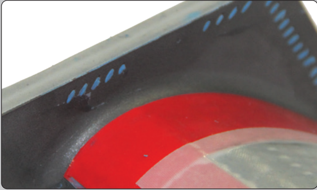
A turbine blade is masked with 170-10S (Red) and 160-5S (White) Masking Tapes as primary and secondary masking. The small cooling holes are filled with HVMC masking compound.
