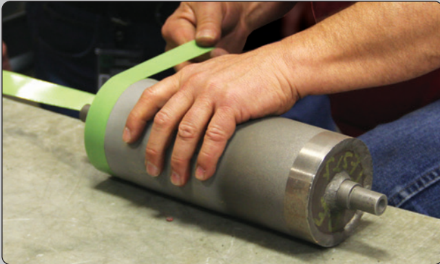
Applying 170-10S Green Masking Tape to a cylinder prior to grit blast and thermal spray coating. Quality tapes like this can stay in place for both grit blast and thermal spray coating.
