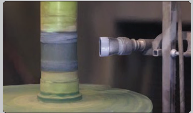
Air cooling reduces substrate temperature and increases masking performance.
