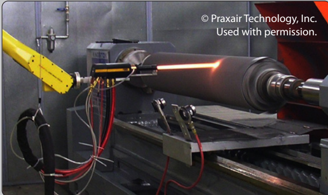
LF-HVOF spray coating is applied to a rotating cylinder.
