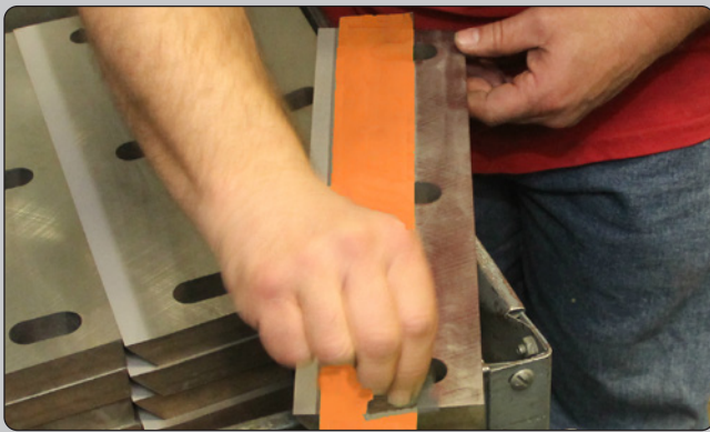
Applying HVMT Orange Masking Tape to a blade prior to receiving coating.
