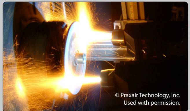
Application of twin wire arc spray at a 90° angle to the target surface.
