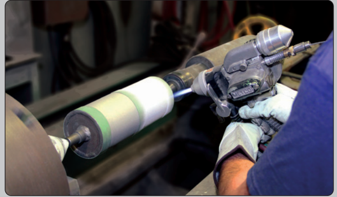
Manual application of combustion spray using a handheld spray gun.
