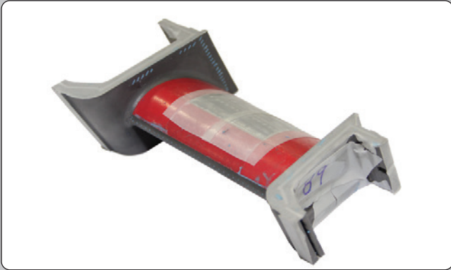
A turbine blade is masked with 170-10S (Red) and 160-5S (White) Masking Tapes as primary and secondary masking.
