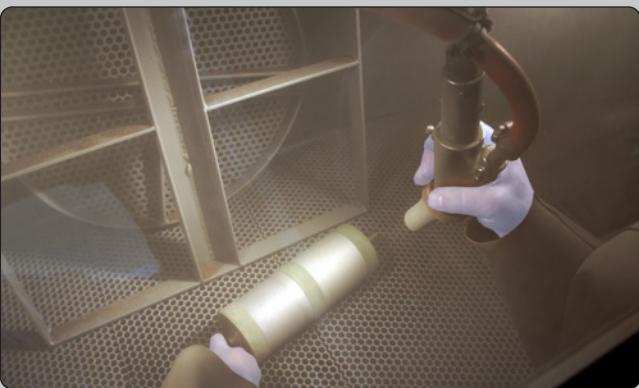
Quality masking products such as this 170-10S (Green) Masking Tape will withstand both grit blast and thermal spray coating processes.
