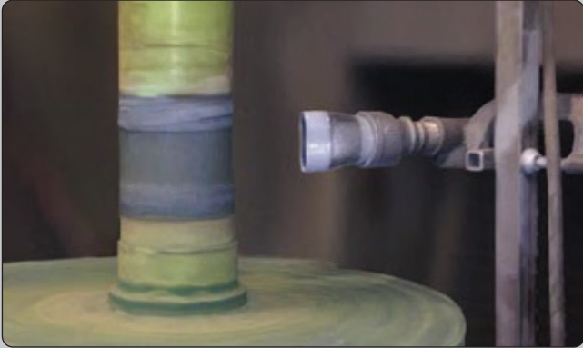
Air cooling reduces substrate temperature and increases masking performance.
